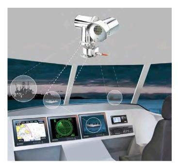
When tracking is disabled, the camera station can be controlled manually by the dedicated touch control panel HERNIS OK160, that provides smooth operation of the Radar Tracking camera and functions.
