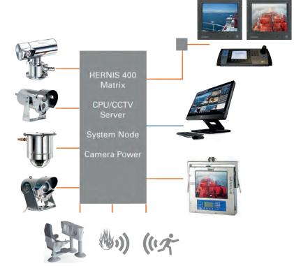
The 400 system matrix may be equipped with audio. A redundant CPU makes the system less susceptible to hardware failures thus improving the systems overall uptime. The HERNIS 400 can easily be upgraded to a hybrid system including both analogue and digital (IP
