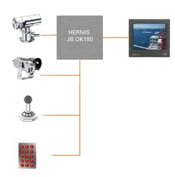
This space efficient solution is perfect where one operator needs visual through one or two camera stations to improve safety and efficiency in operations. The JB OK 150 serves as a control unit for the camera stations.
